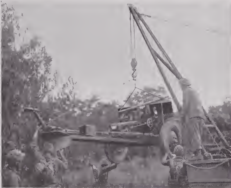
FIGURE 13. During OSRD-initiated demonstration at Milne Bay, New Guinea, U. S. Marine Corps artillery is unloaded from one DUKW by another DUKW equipped with A-frame.
